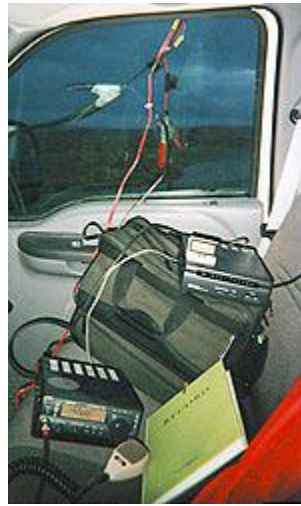
Amateur Radio station KL7JR, as set up in the temporary mobile operating position from the job office area on Shemya Island--note the jumper cables running into the cab through the window.
