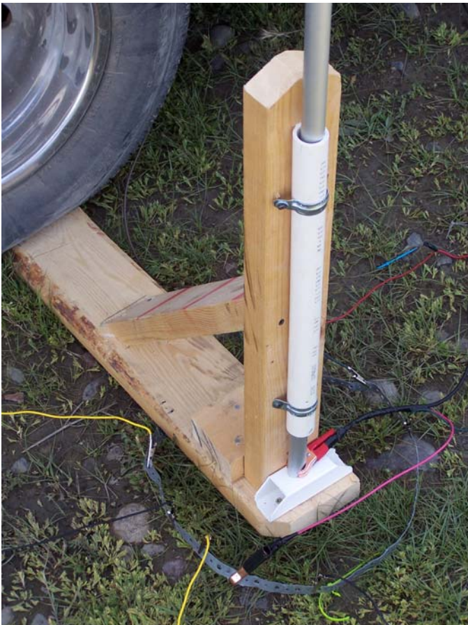
Quickie homebrew base from scrap lumber with ground ring and coax connections.
