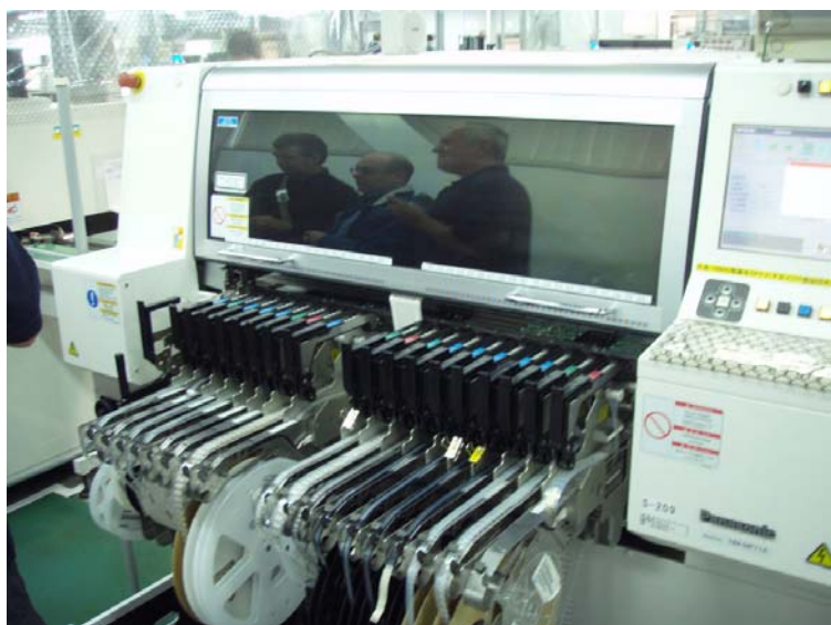
Machine assembling circuit board from components on Mylar tap cartridges.
