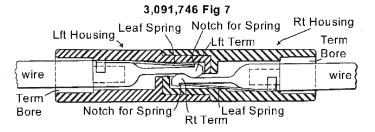
Also, in the two newest patents, each side of the housing has a dovetail groove or tongue so you can stack the housings side by side and/or top to bottom. There may be as many as 12 different ways to connect two housings. ARES has standardized a pairing scheme for a red and a black housing for use with common "12 Volt" equipment using either the 15 Amp or the 30 Amp contacts.
