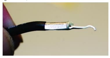
Note that the end of the crimped portion has slightly bunched up. This is not a properly crimped pin.
