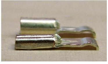
The contact in the foreground has been crimped. The "spoon" component of the contact extends in a straight line; this angle must be maintained for proper mounting of the housing. If they are bent slightly upward they may not stay in the housing; bent down they do not mate with full force.
