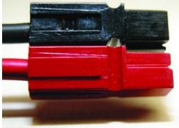
Tongue-and-groove dovetailing in the connector housings allows the cases to be connected snugly to each other.
