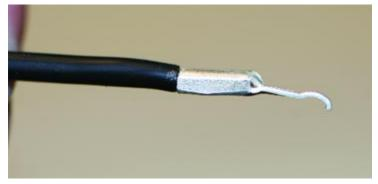
This pin has been crimped; notice that the contact portion has been bent slightly downward in the crimping process. A slight downward or upward bend can occur depending on the wire size you are using for a given pin. This is normal—the secret is to bend the pin back to align it parallel with the crimped
