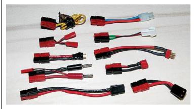
You are already using other connector types? No worries, you can quickly and easily make patch cords to ensure cross compatibility for all your electric flight options. You can easily make parallel circuit patch cords (for flying with 2P lithium setups), and you can easily connect two batteries in series using Powerpoles. Few connector systems offer the ease of use of Anderson Powerpoles.
