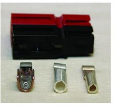
for 10–14 gauge wire; the "30 amp" pin (#1331) is for 12–16 gauge wire; and the "15 amp" pin (#1332) is for 16–20 gauge wire. Once installed in connector housings, these different size pins snap together perfectly on the contact side.
