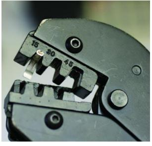
If a pin "sticks" in the upper seat of the crimping jaw and you open the crimper fully, the die cavity will bend the front of the pin down, as shown, which will likely ruin the pin.
