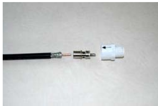
Use a step drill and ream out the female end.
