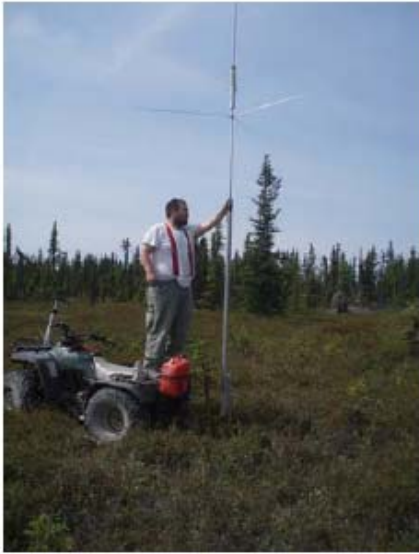
Muskeg near the sea with radials make for a hot vertical ground plane on 75 meters. (Photo - Kris Kerce AL2F)
