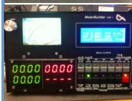
Pic 13: As above, note dashes are SWR meter, currently dashes indicating no reading.
