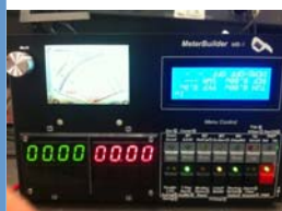
Pic 7: Power on! This caused an issue which, if you look, the LCD is installed upside down. This caused the issue where it beeps warning you of a fault.
