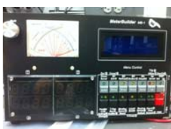
Pic 7: Power on! This caused an issue which, if you look, the LCD is installed upside down. This caused the issue where it beeps warning you of a fault.
