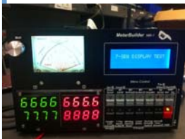
Pic 10: Part of self test routine doing 7-segment LED display
