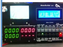
Pic 12: Powered up and ready for use. Initially, bottom 2 7-segment displays are turned off. Easily fixed in menus.
