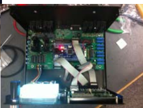
Pic 10: Part of self test routine doing 7-segment LED display
