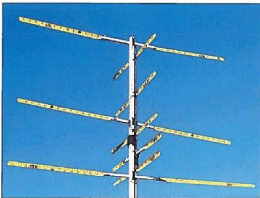
Figure 1 — Dual purpose, dual boom portable tape measure Yagi for 2 meters and 70 cm.
